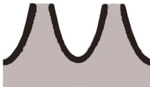
Quenching of Tooth Surface and Dedendum
